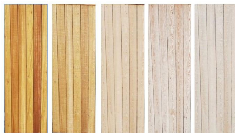
Fig. 12 - A natural timber species showing varying rates of weathering over 7 months, the final result is a silver-grey nuance (Britton Timbers, 2020)
