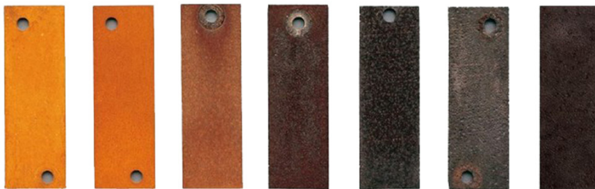
Fig. 11 - The weathering of steel over time (The Nippon Steel Corporation, n.d.)
