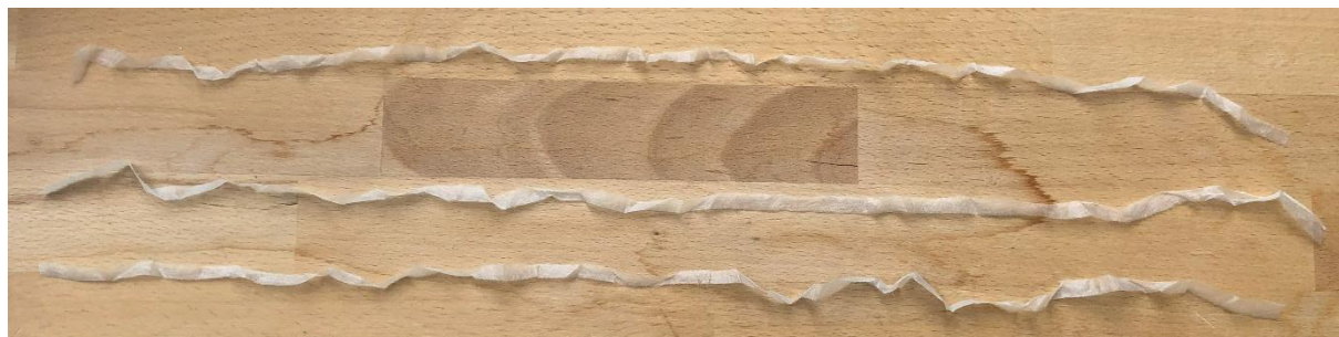
Figure E4: Top sheet samples for determining the weight of the top sheet.
