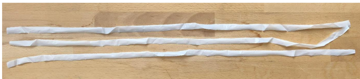
Figure E3: Bottom sheet samples for determining the weight of the bottom sheet.
