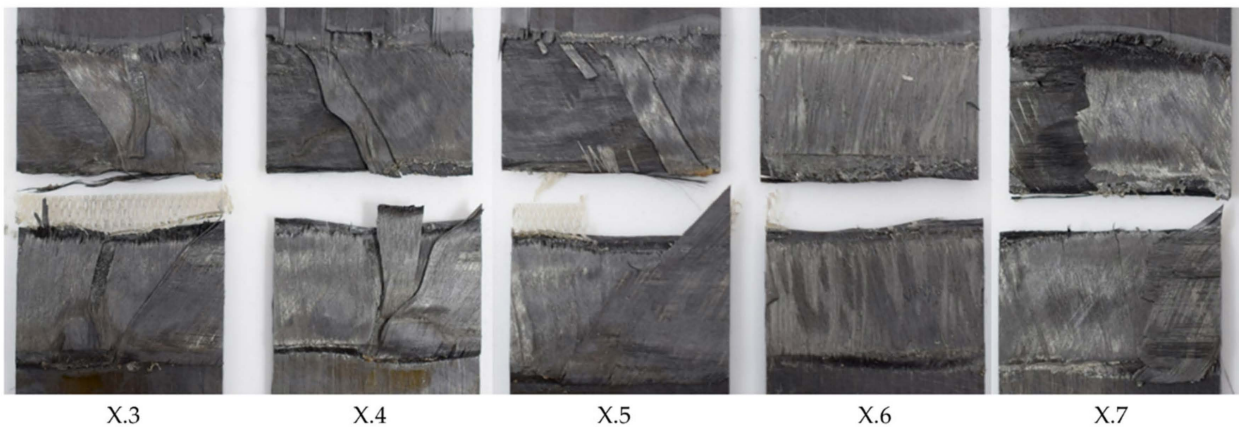
Figure 14. Fracture surface of sample welded with 100% amplitude and 16 mm/s welding speed using the thin energy director (samples X.3–X.7 from left to right). The fracture surface shows failure mostly in the 135° ply and fibre misalignment.
