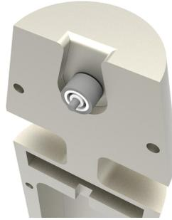
Figure 5.7: Cut-open view of the cavity in the satellite's rear for storing the Hyperflo cable.
