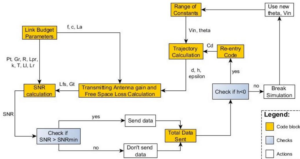
Figure 7.2: Flow diagram of the link budget analysis program.
