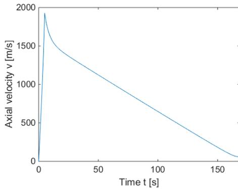
Figure 6.3: A plot of the axial velocity versus time during ascent.
