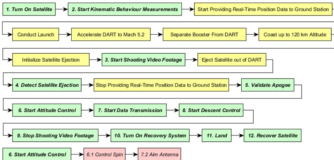
Figure 2.3: Functional flow block diagram of the mission.
