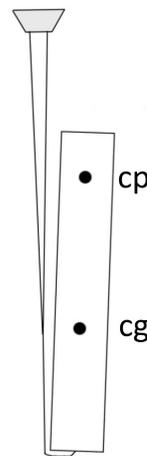
Figure 6.18: Tubesat with a cg higher than cp has risk of flipping around.
