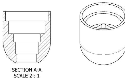
Figure 5.5: Nose cone design.
