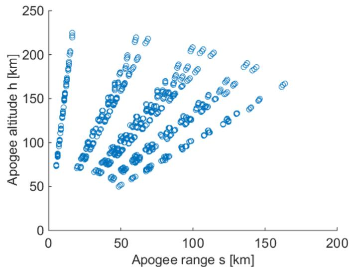
Figure 10.1: A scatter plot of the apogee altitude and -range for all parameter combinations.
