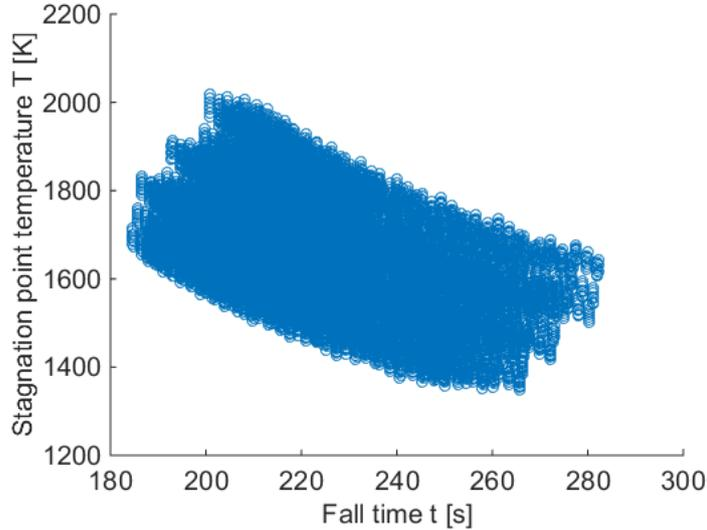
Figure 10.2: A scatter plot of the stagnation point (equilibrium) temperature and fall time for all parameter combinations.
