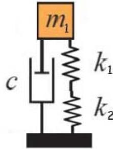
Figure 9.1: Discretization of the TubeSat.
