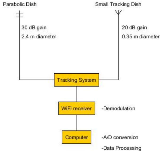
Figure 7.6: Lay-out of the WiFi ground station.
