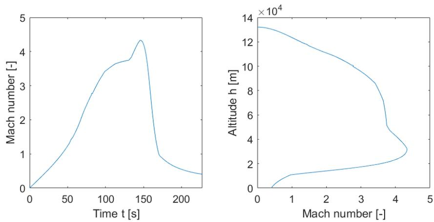
Figure 6.11: Plots of the Mach number versus time and altitude during descent.
