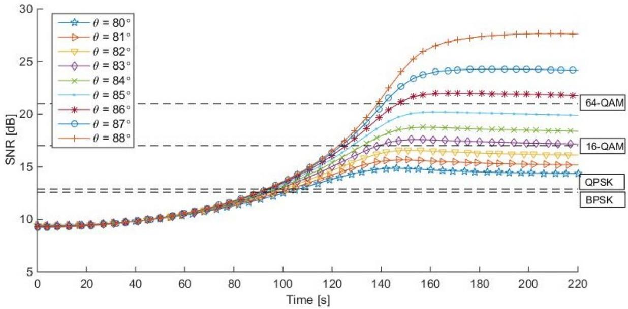
Figure 7.7: The SNR over time for different launch angles for WiFi.
