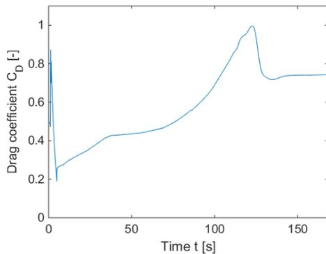
Figure 6.5: A plot of the drag coefficient versus time during ascent.
