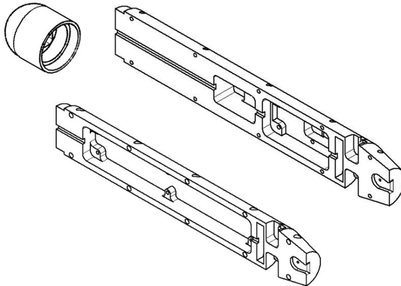
Figure 5.3: Overview of the outer shell of the satellite.
