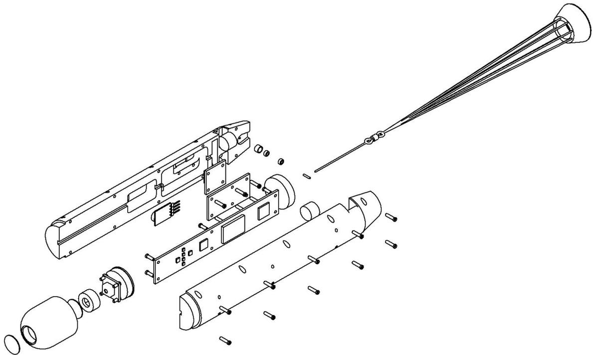
Figure 12.16: TubeSat exploded view.
