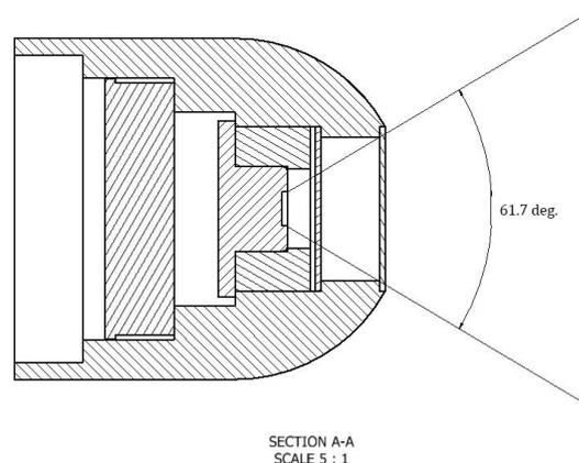
Figure 5.4: Angle of view of the camera.
