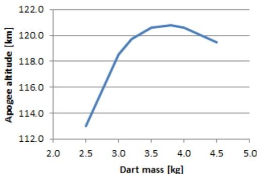
Figure 11.1: The influence of the total dart mass on apogee altitude. A courtesy of TME.
