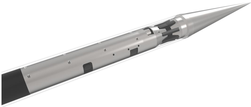
Figure 5.16: Overview of TubeSat in the dart before launch.
