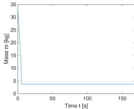
Figure 6.6: A plot of the rocket mass versus time during ascent.
