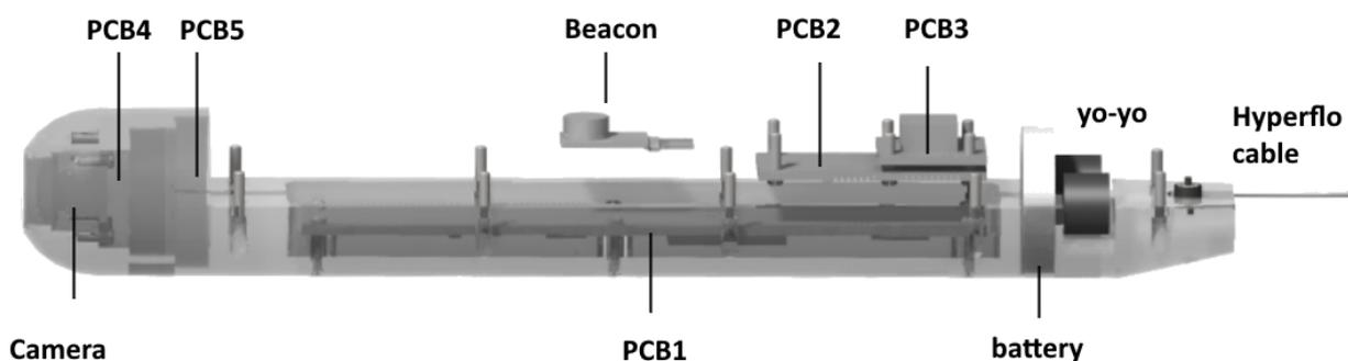
Figure 5.2: Overview of the layout of the satellite's inside.
