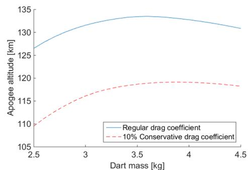
Figure 11.2: The influence of the total dart mass on apogee altitude. Launch simulation results.
