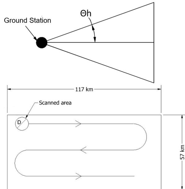
Figure 7.5: Horizontal scanning angle sketch and 2D plane that needs to be scanned.
