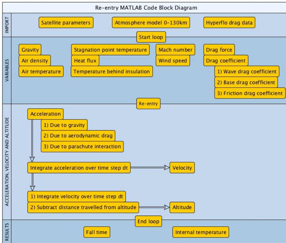
Figure 6.8: A block diagram of the MATLAB re-entry code.
