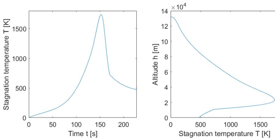
Figure 6.15: Plots of the stagnation point temperature versus time and altitude during descent.
