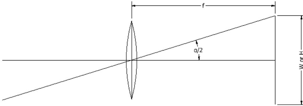
Figure 5.9: An overview of the lens-sensor system.
