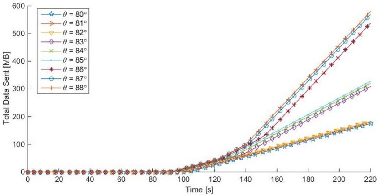
Figure 7.8: The amount of data sent over time for different launch angles for WiFi.
