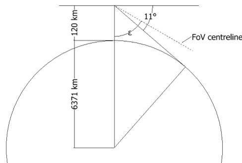
Figure 5.8: An overview of the view angles at apogee (drawing not to scale).
