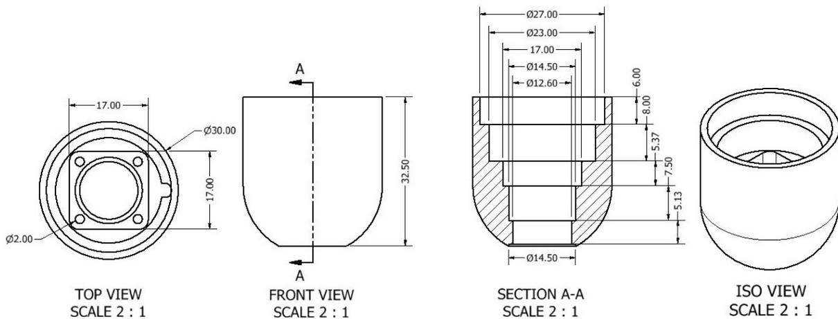
Figure 12.4: Nose cone production.
