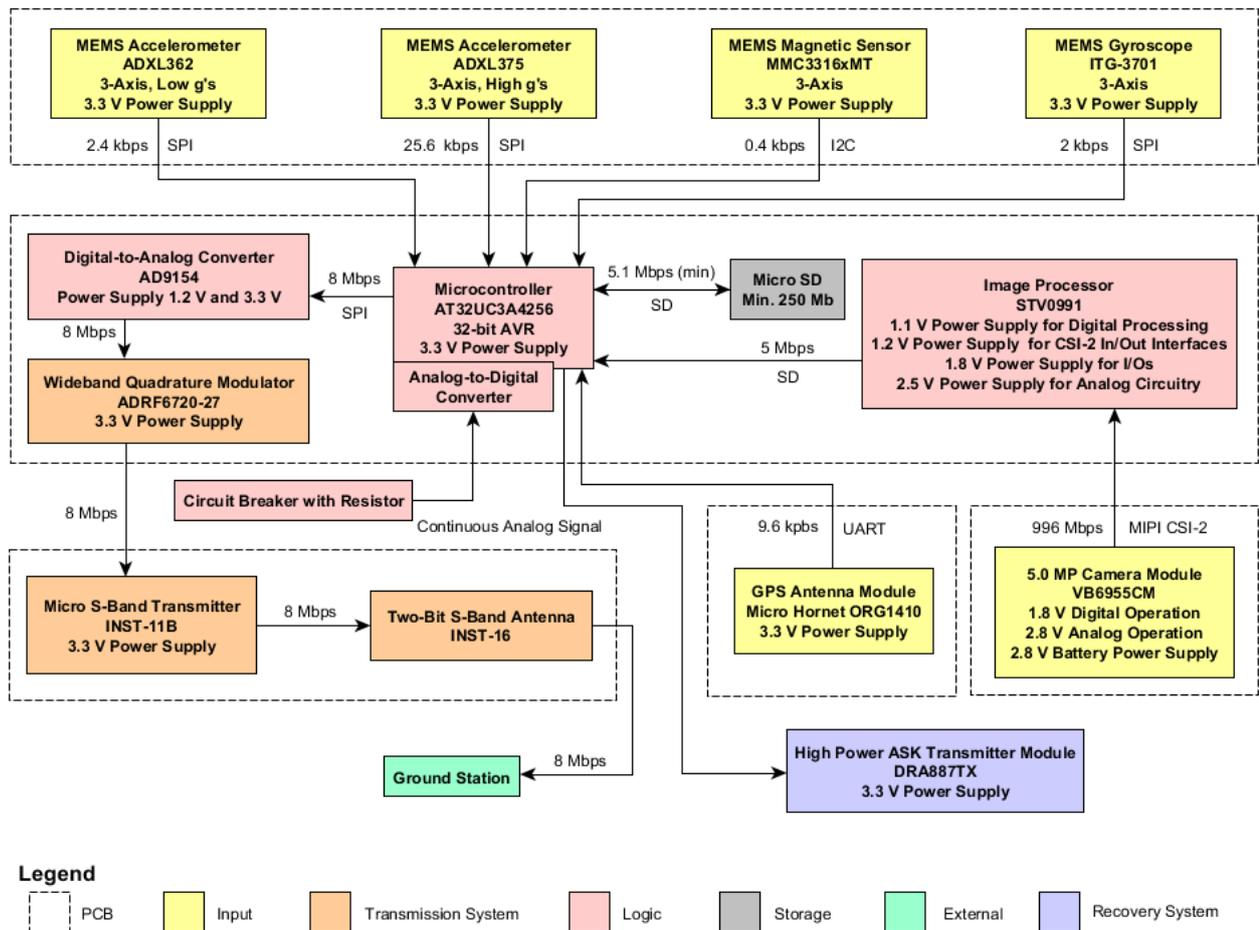
Figure 8.4: Data handling block diagram.
