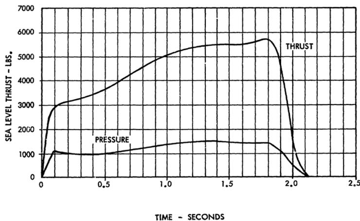
Figure 11.3: Variation of Super Loki sea level thrust with burn time.
