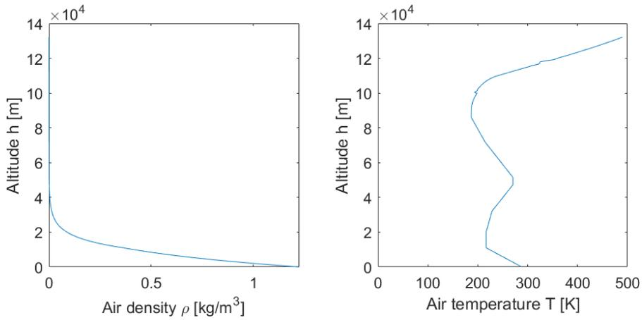
Figure 6.13: Plots of the air density and air temperature versus altitude.
