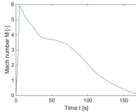
Figure 6.4: A plot of the Mach number versus time during ascent.
