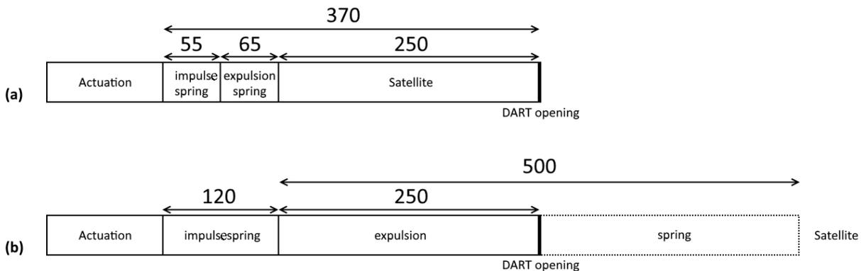
Figure 5.10: Spring dimensions in TMEs design.
