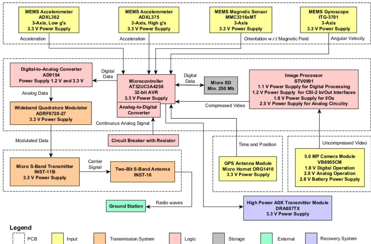
Figure 8.5: Software block diagram.
