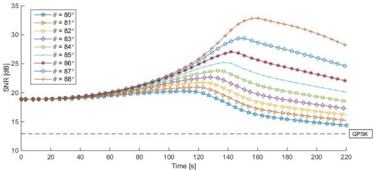
Figure 7.3: The SNR over time for different launch angles for the transmission at ESC.
