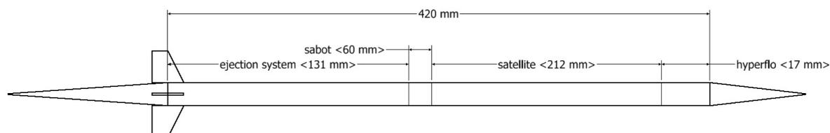
Figure 5.1: Overview of components inside the dart (not to scale).
