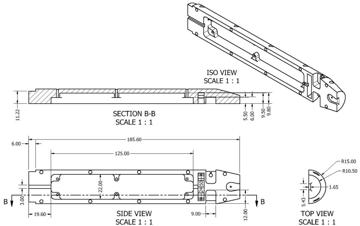
Figure 12.3: Right outer shell production.
