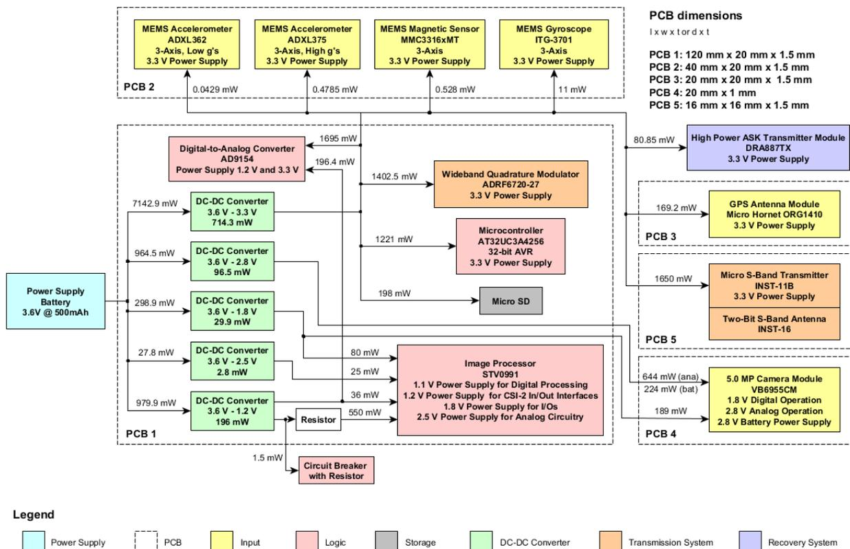
Figure 8.1: Electrical block diagram (ana = analog, bat = battery).
