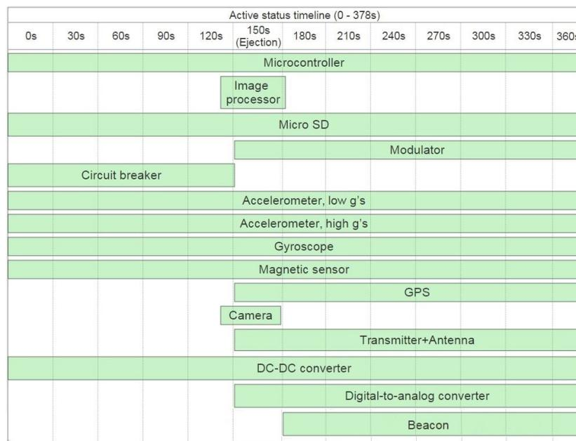
Figure 8.2: Active status timeline of electrical components.
