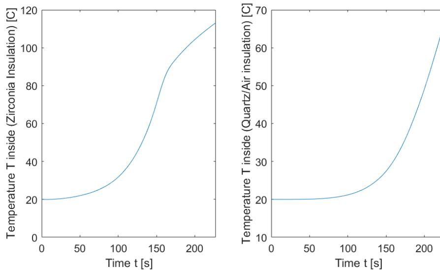
Figure 6.16: Plots of the temperature behind the insulation versus time during descent.
