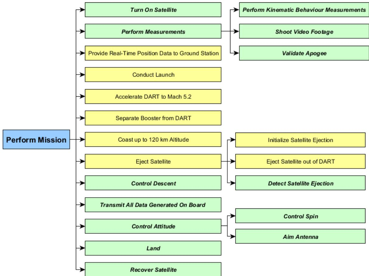
Figure 2.2: Functional breakdown structure of the mission.
