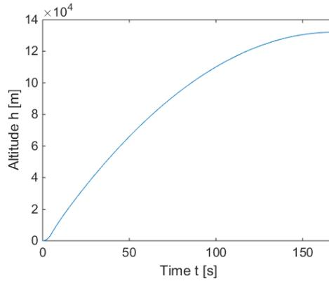
Figure 6.2: A plot of the altitude versus time during ascent.
