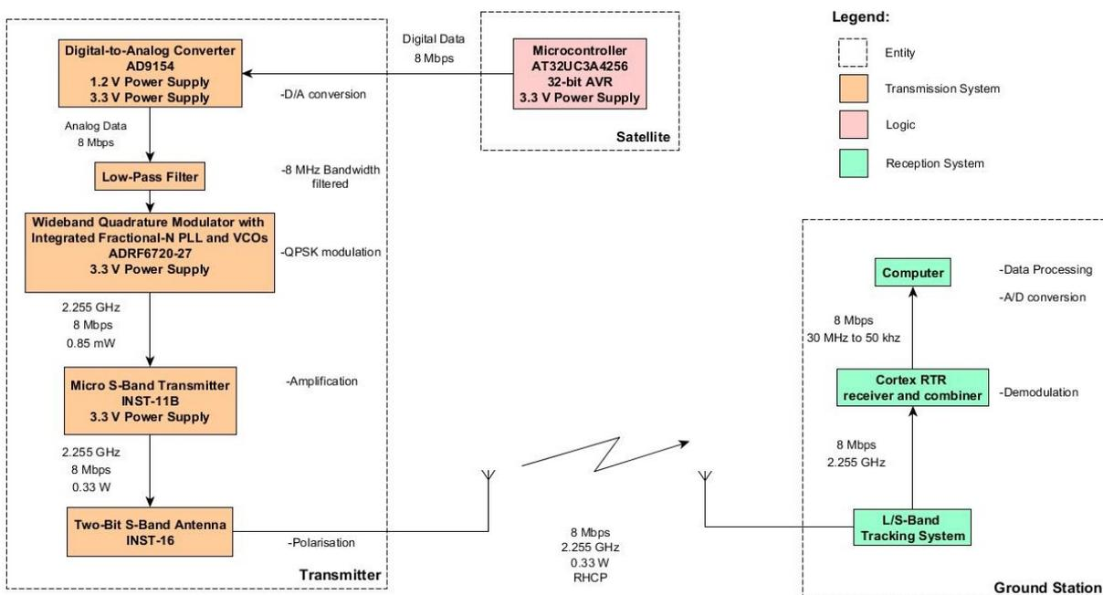
Figure 7.9: The communications flow diagram with the ESC ground station.
