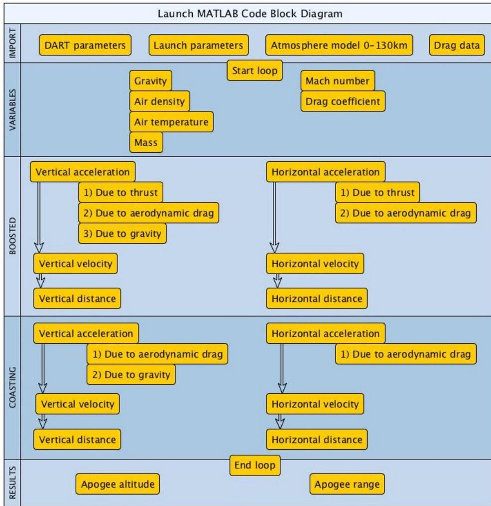
Figure 6.1: A block diagram of the MATLAB launch simulation code.
