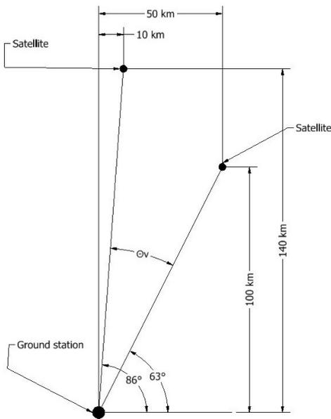
Figure 7.4: Vertical scanning angle sketch.
