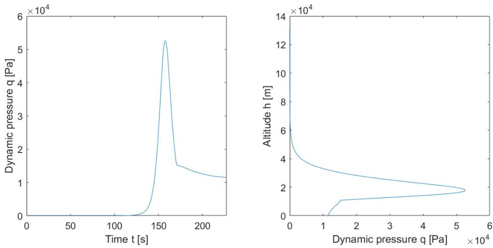
Figure 6.14: Plots of the dynamic pressure versus time and altitude.
