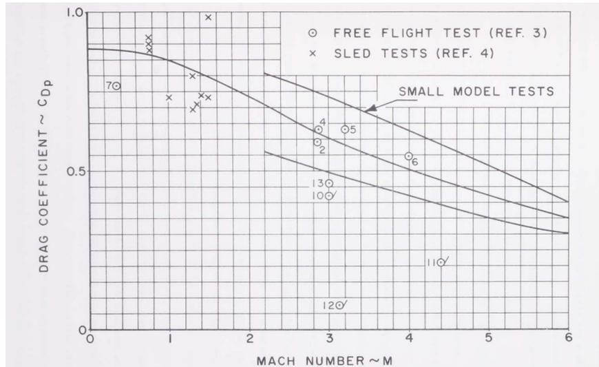
Figure 6.7: Variation of hyperflo drag coefficient with Mach number [50].
