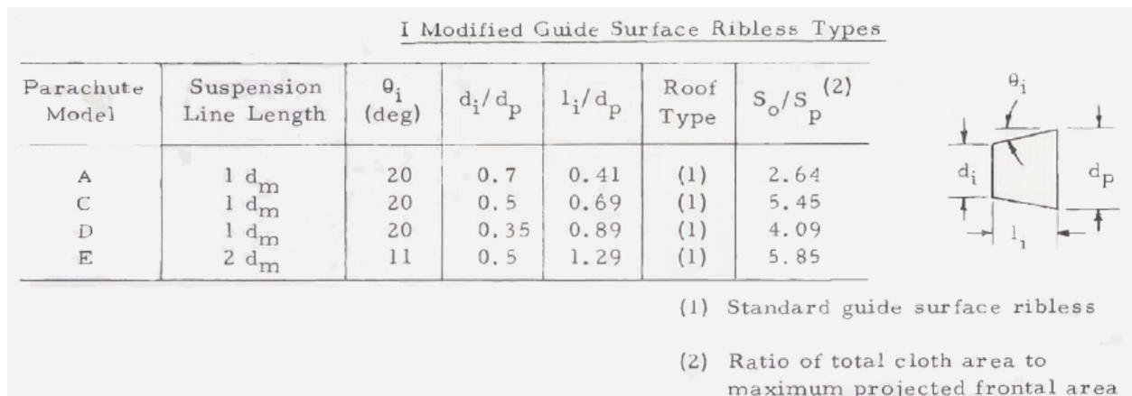
Figure 5.13: Schematic overview of hyperflo geometries in the Phase I tests [51].
