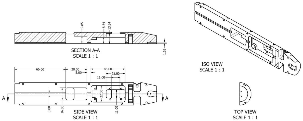
Figure 12.2: Left outer shell production.
