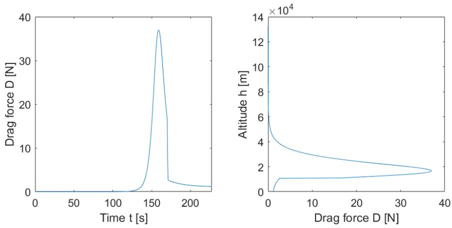
Figure 6.12: Plots of the satellite drag force versus time and altitude during descent.
