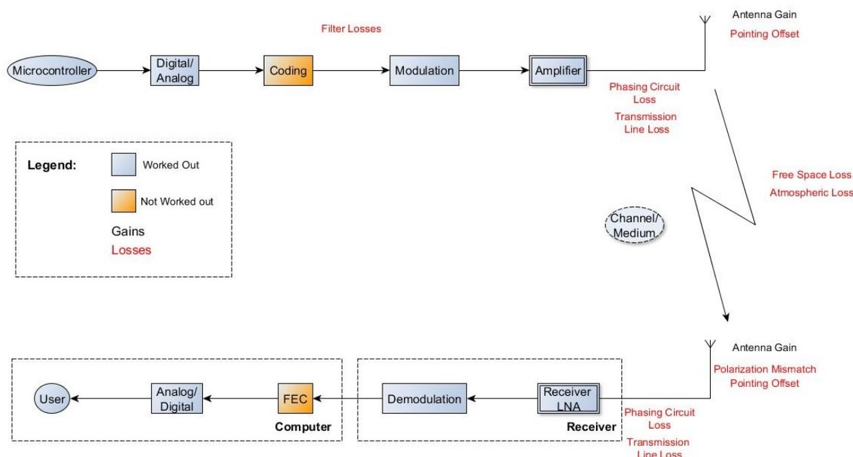
Figure 7.1: The general lay-out of a communication system.
