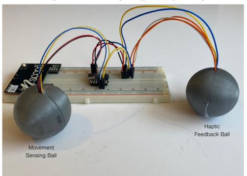
Figure 45. Rotation/Movement Prototype Assembly
