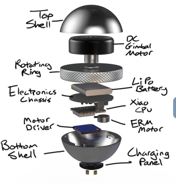
Figure 50. Labelled Exploded View of Fidget Sphere, own image.
