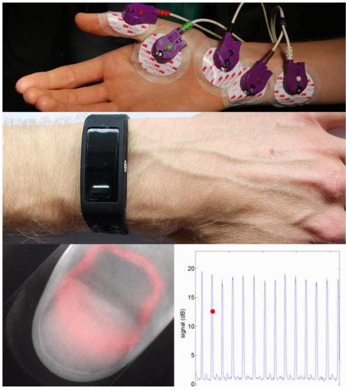
Figure 21. Composite Visual for Biosensing Technologies. Top: EMG, Middle: PPG Wristband, Bottom: Laser Doppler Imaging of BVP of Thumb
