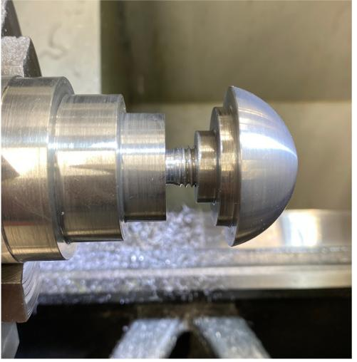
Figure 54.Hemisphere Body Being Screwed On Custom Lathe FixtureFigure 55.(Next Spread) Fidget Spheres Looks Like Prototype with Stand
