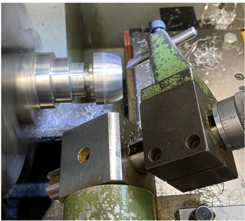
Figure 56. Sphere Rounding Process
