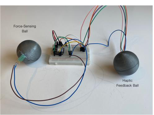
Figure 44. Force Sensing Prototype Assembly, own image
