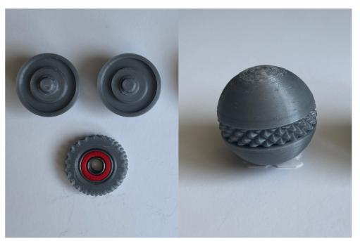
Figure 37. Spinning Ring Prototype with ABEC Bearing
