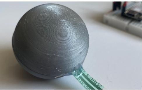
Figure 39. PLA 3D Printed Shell of Prototype Fidget Sphere
