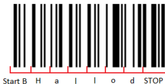
Figure 5.12: The interpretation of a Code-128 barcode as generated by our custom interpreter.
