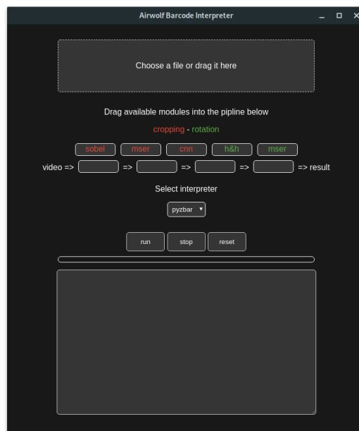
Figure 5.11: Our Electron based Graphical User Interface. The top shows the drag-and-drop field to place the video file, below that is the pipeline with available modules and below that is the output field with start, stop, and reset buttons.
