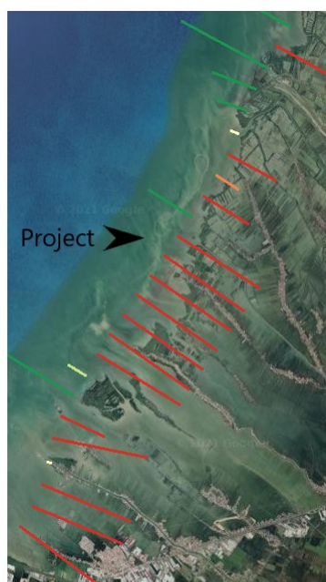
Figure 1.3: The red bars present erosion (3 m/yr or more) and the green bars present accumulation of sediment (3 m/r or more).The retreat of the coast in the period of 1985 - 2016 in the Aquamonitor available via https://aqua-monitor.appspot.com/?datasets=shoreline .
