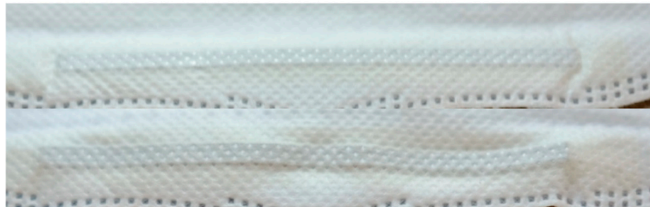
Figure 7. Nose clip after usage showing wavy pattern (Top: unused filtering facepiece respirator (FFR), Bottom: used FFR brought back to neutral position).
