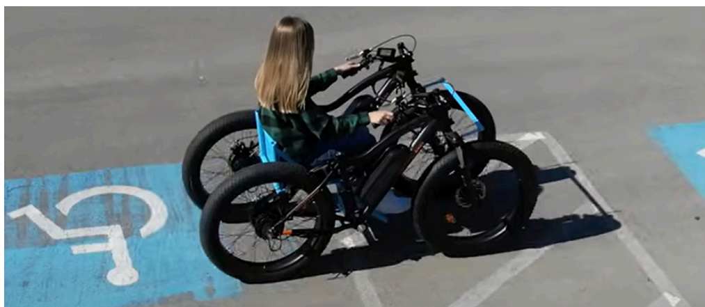
Figure 24. Off-road wheelchair constructed from two electric bikes by a YouTuber (JerryRigEverything, 2018).
