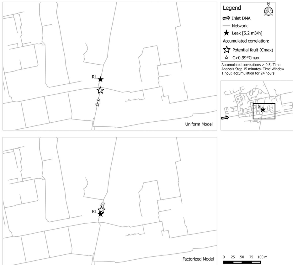
Figure 2. Highest accumulated correlations in the uniform (top) and factorized model (bottom) from the real leak.
