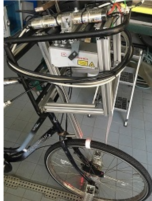
(b) Close up laser setup on bicycle.
