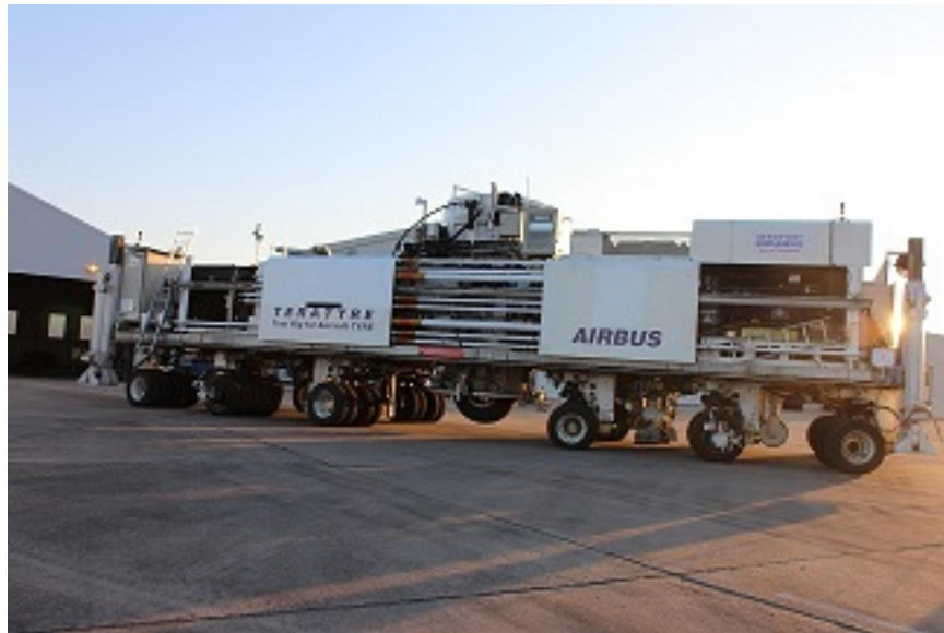
Fig. 8 Test Rig for Aircraft Tires (TeraTyre) at Châteauroux Airport with in the centre the aircraft tire being tested.
