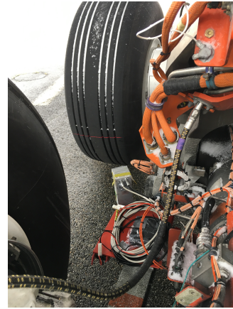
(b) Profilometer system cradle on left main landing gear outboard brake strut.
