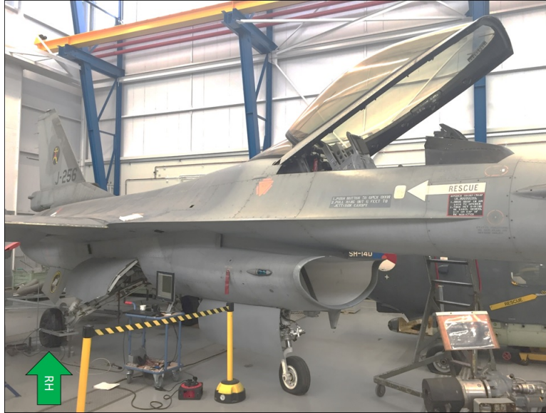
Fig. 3 F-16 profilometer Ground Test, main landing gear tires (right hand main wheel shown with green arrow).
