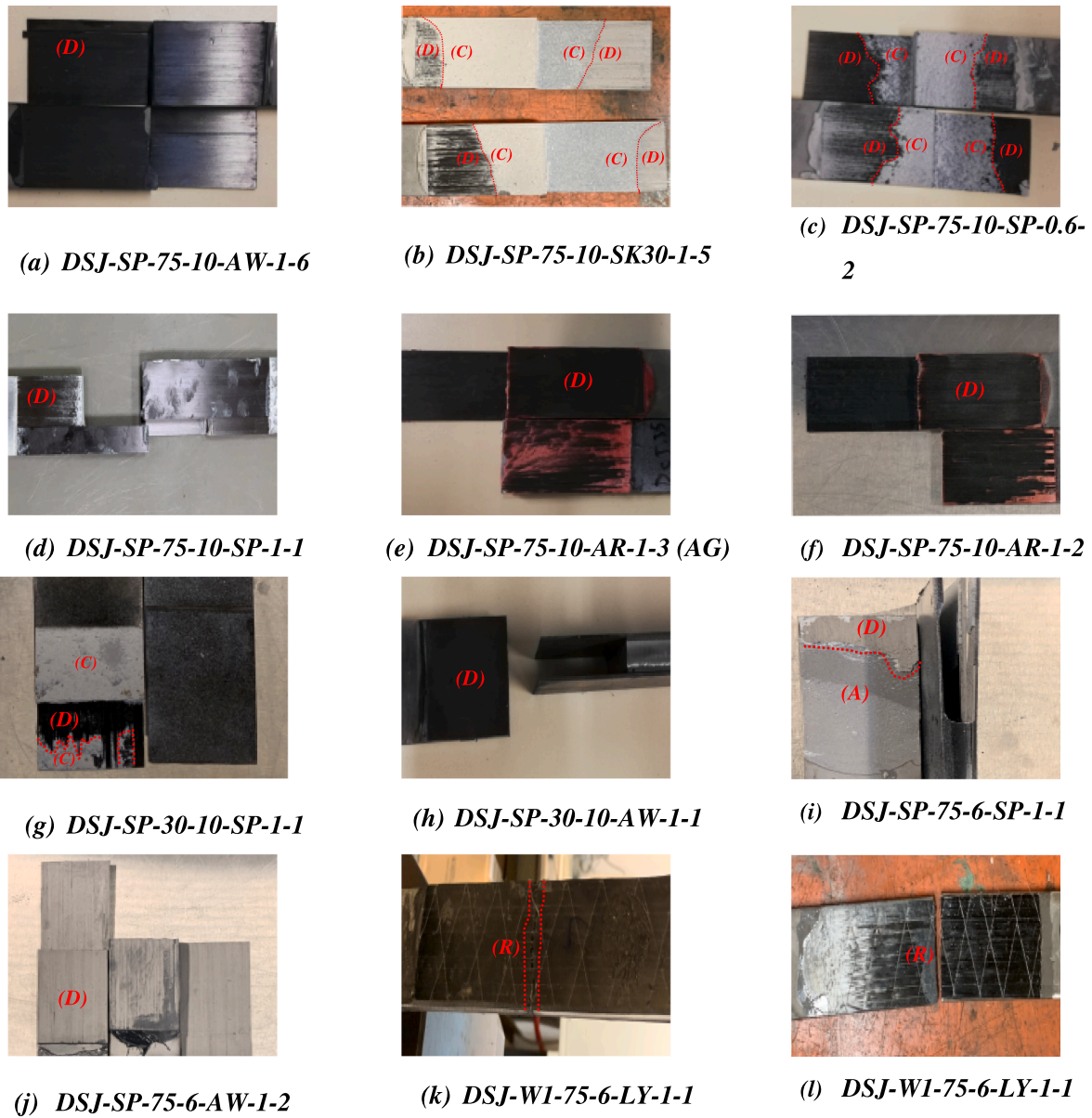
Fig. 6. Observed failure modes.
