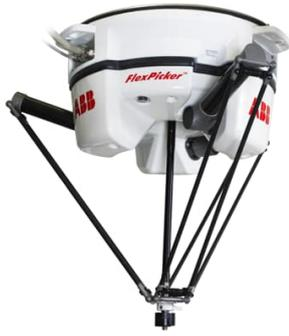
Fig. 4: FlexPicker Delta robot by ABB [3].
