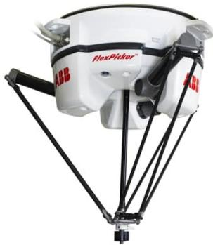
Figure 1.1: Delta robot by ABB.
