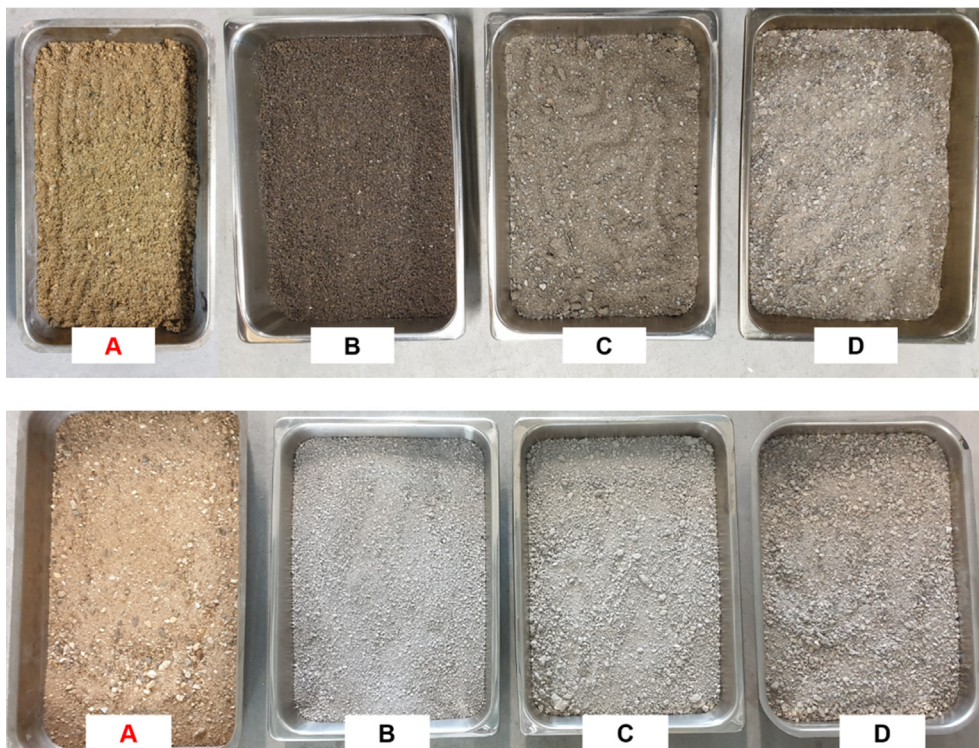
Fig. 1. River sand and fRCA before (top photo) and after (bottom photo) drying (river sand (A) and fRCA with different origins (B, C, D)).
