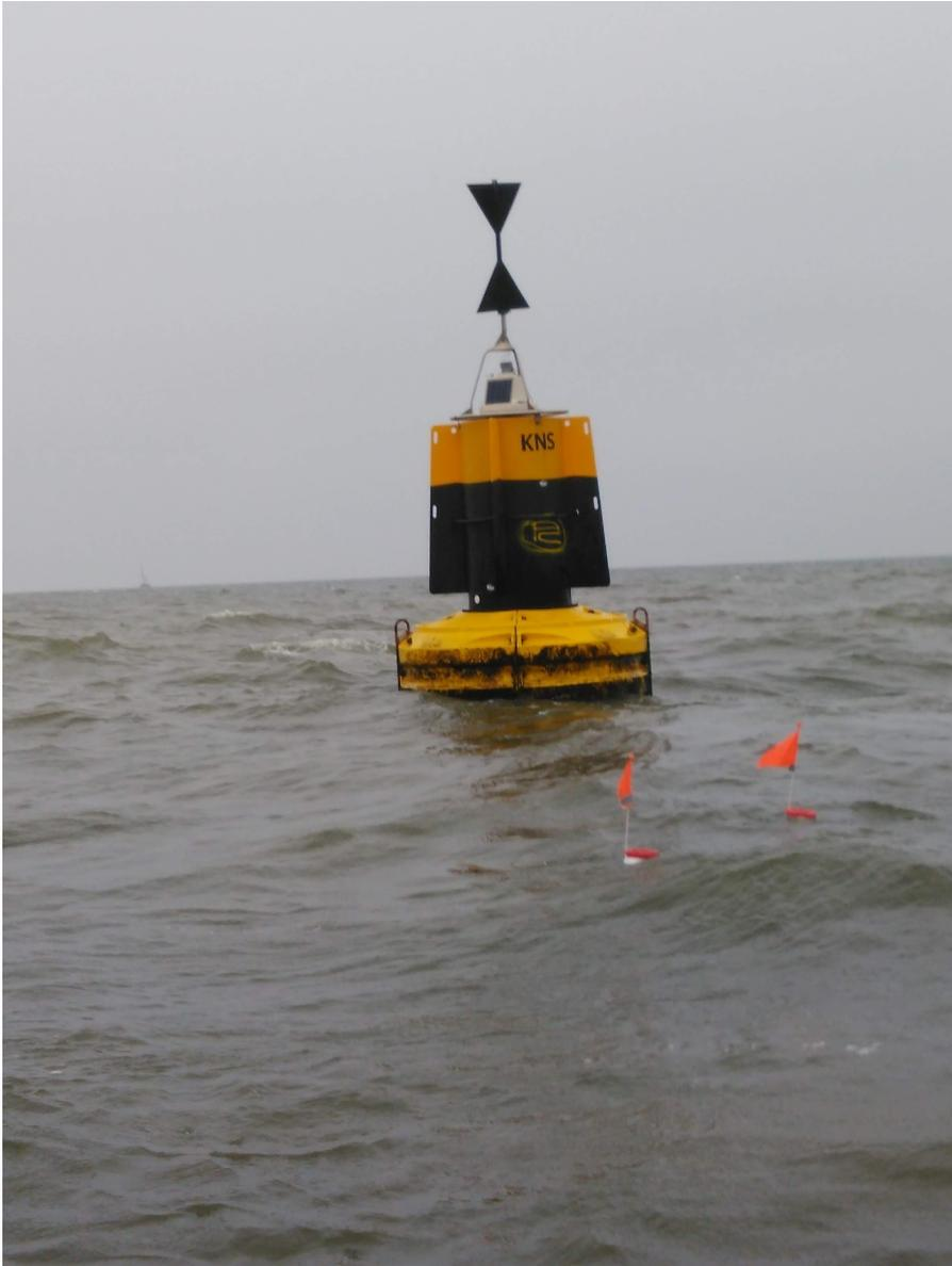
Figure 46: Two of our buoys (orange flags) drifting freely near Scheveningen harbor in the Netherlands. The larger buoy, de Kardinaal, is chained to the ocean floor. The smaller buoys are equipped with ublox-neo m8t single frequency GNSS receivers. The antenna is from Taoglass of type Magma X AA.170.
