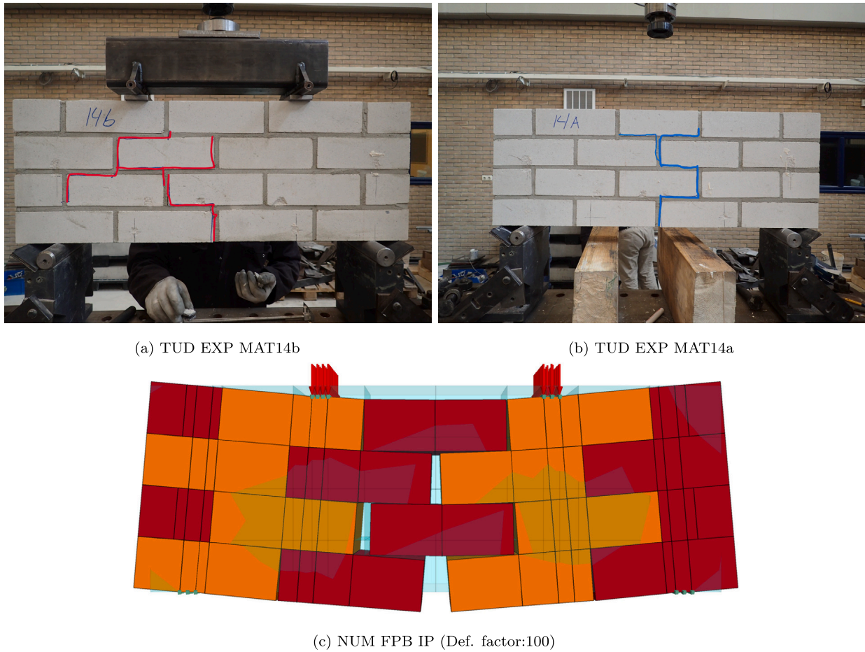
Fig. 14. Comparison of (a), (b) experimental crack pattern and (c) numerical deformed shape (magnified 100 times).
