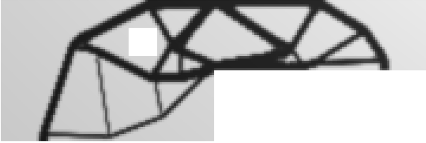
Figure 3.3: Optimized topology of the dapped-end beam. Black and grey pixels indicate the solid and void regions.
