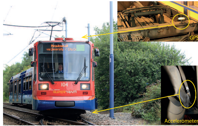
Figure 3. ABA system used with close-ups of the GPS antenna and an accelerometer
