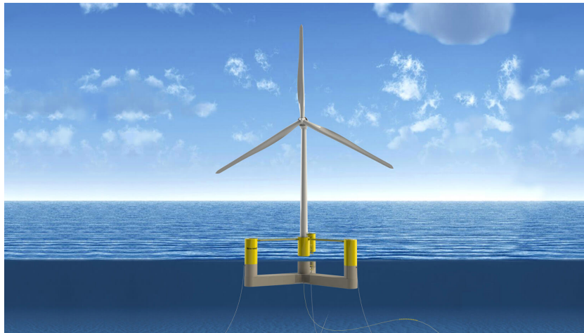
Figure 3.7: The UMaine VoltturnUS-S reference platform[39]
