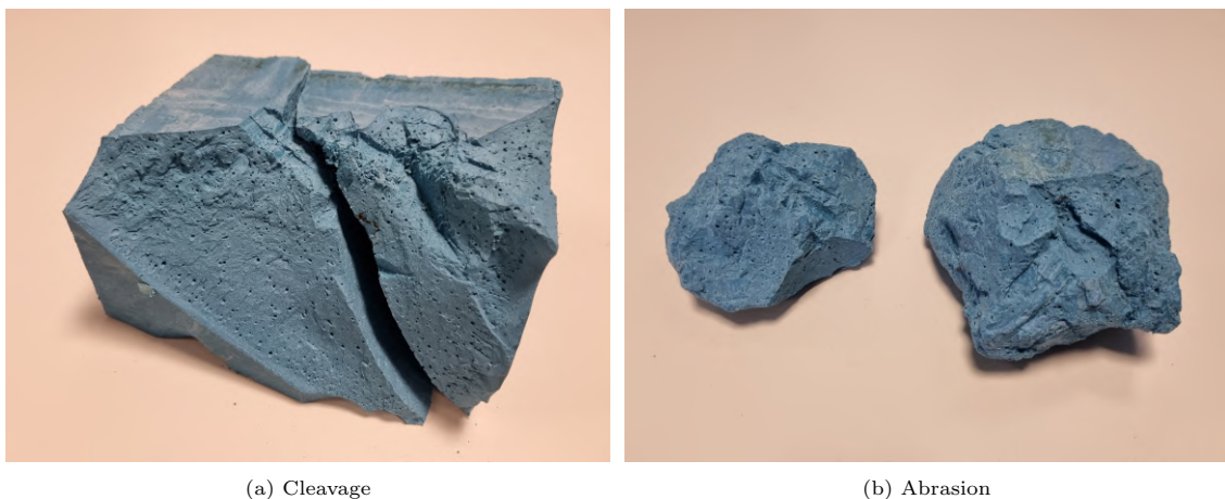
Figure 4: Examples of breakage mechanisms
