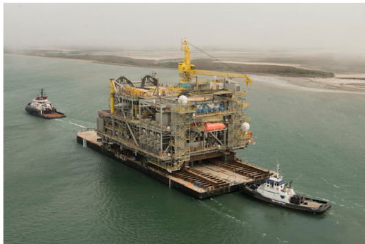
(c) Tug Barge System
