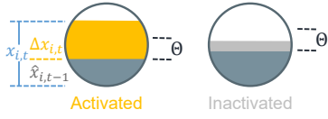
(a) Delta neuron is activated when the activation change |\Delta| exceeds the delta threshold \Theta at a certain timestep.
