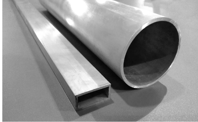
Fig. 15. Extruded magnesium alloy tubes.
