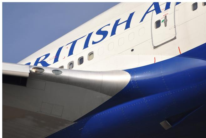
**Figure 1.11:** Picture of leading edge fairing on a commercial Boeing 747.
