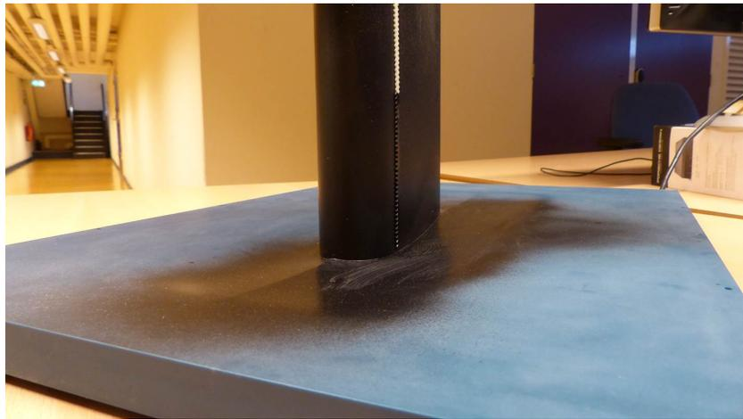
**Figure 3.5:** Photograph of the antifairing with Rood wing installed.
