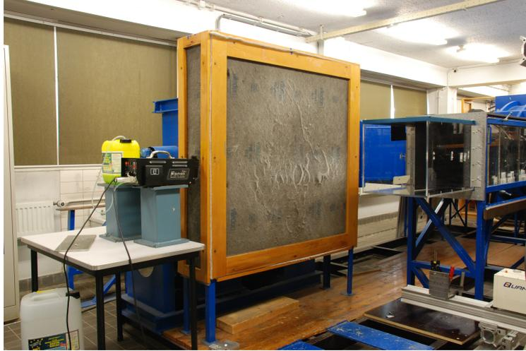
**Figure 3.1:** Picture of the M-tunnel. Fog generator and wing tunnel inlet on the left and test section on the right.
