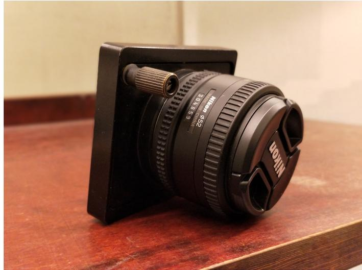
**Figure 2.6:** Picture of a Scheimflug adaptor with lens attached.
