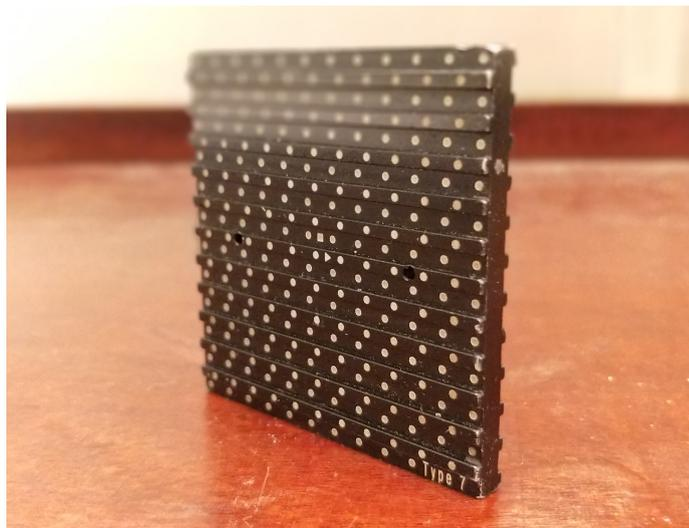
**Figure 2.7:** Calibration plate used in the current sPIV study.
