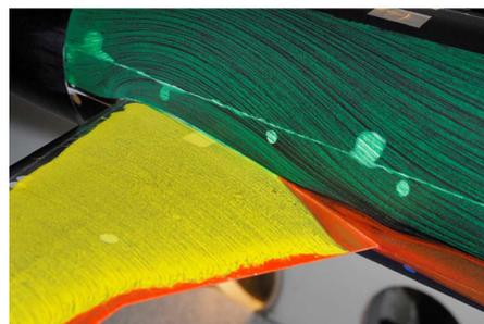
**Figure 1.2:** Oil flow visualization of DLR F6 model at wing-fuselage junction ([Rudnik et al., 2009](#)).
