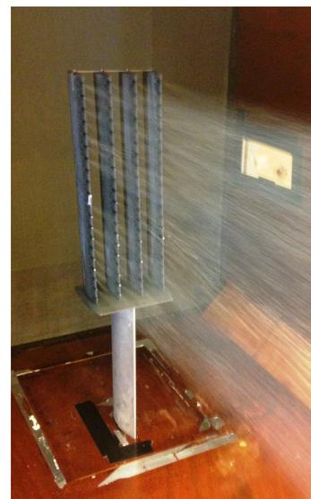
**Figure 1.14:** Seeder in operation installed inside a wind tunnel. Image from Jux (2017).
