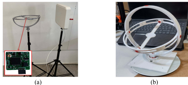
Fig. 3. Fabricated Open Gimbals for (a) Tripod and (b) Tabletop version along with the sensing system and sensor PCB.
