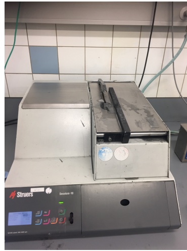
(b) Diamond precise abrasive cutting machine
