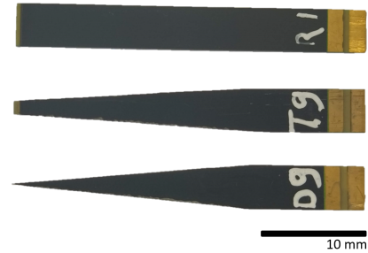
Fig. 1: Three bimorph tapered piezoelectric cantilevers shaped by abrasive water cooled cutting for reliability and power output experiments.
