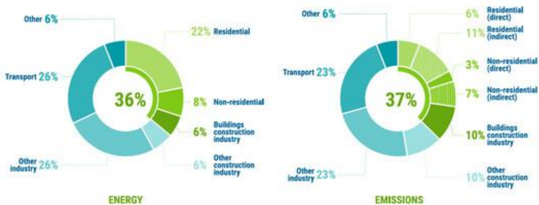
Figure 6 Construction Industry's Share of Global Final Energy and Energy-Related CO2 Emissions (UNEP, 2021)
