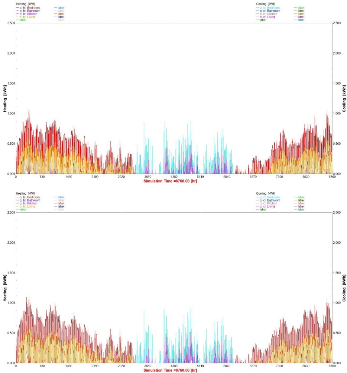
Figure 89 Studio- Annual Heating Cooling Energy flux, Hybrid (above) and WFO (below) (Author, from TRNSYS)
