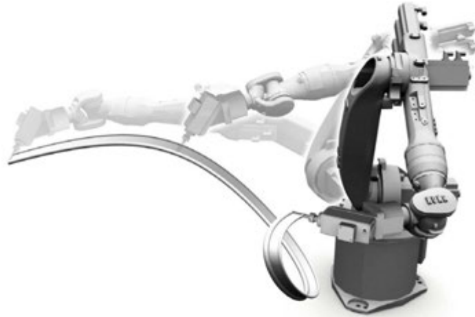
Figure 1.10: A 6-axis articulated robot tracing a free-form curve with a milling cutter
