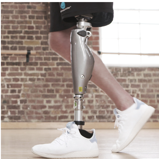
(a) The C-leg prosthesis [4]
