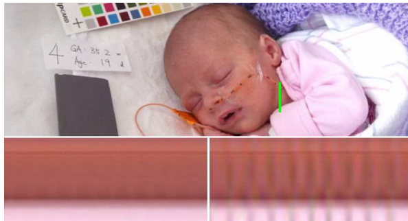
Figure 3: Intensity magnification on a static video. We indicate with a green stripe the locations at which we temporally sample the video. Note that our method is well able to magnify the intensity for videos without large motions.
