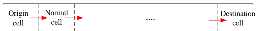
Figure 6.1: The depiction of cells and links. Red arrows represent links, and black dashed lines represent the boundaries between cells. Origin cells have no incoming link and destination cells have no outgoing link. Normal cells are connected by one incoming link and one outgoing link.
