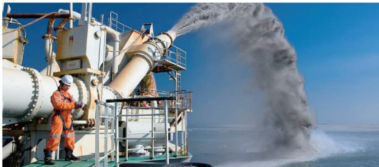
Figure 2.21: The rainbowing method of placement (Van't Hoff & Nooy van der Kolff, 2012)
