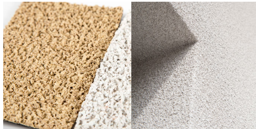
frame: cork plaster spray
