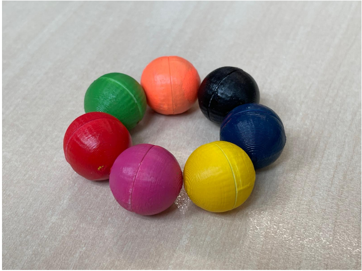
Figure 5.10: Printed magnetic spheres in seven different colours
