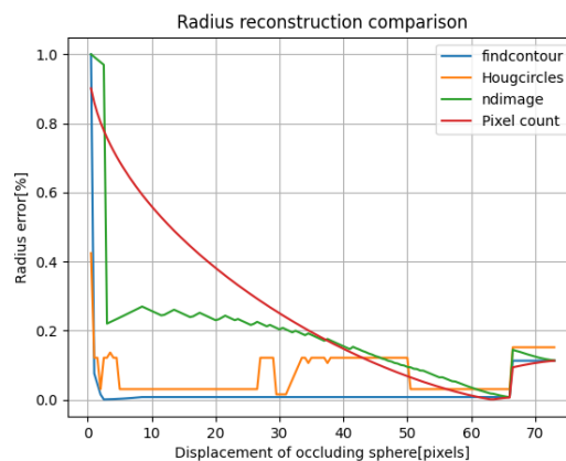
Figure 6.8: Comparison of radius reconstruction when displacing one occluding sphere
