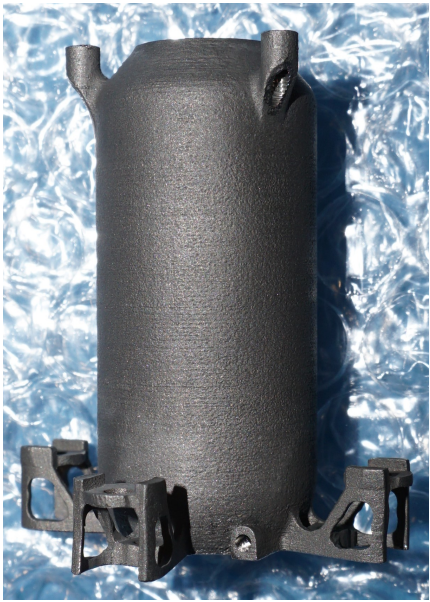
(a) 3D printed heating chamber after printing and machining of holes and (b) 3D printed heating chamber cut in half via EDM for internal inspection
