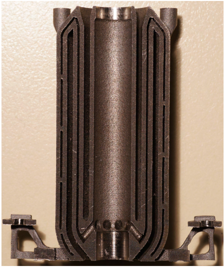
(a) 3D printed heating chamber after printing and machining of holes and (b) 3D printed heating chamber cut in half via EDM for internal inspection
