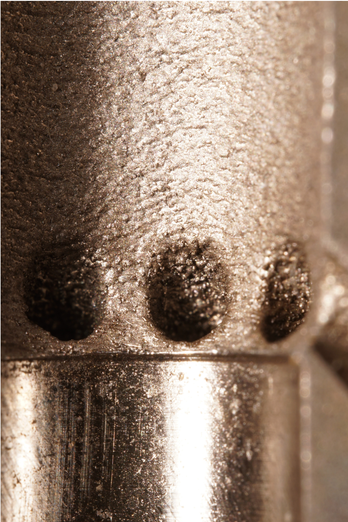
Figure B.5: Close up picture showing the surface roughness of the channel walls of the as printed part
