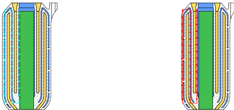
(a) Heating chamber section cut view with flow path highlighted by light blue arrows (b) Heating chamber section cut view with heat conduction path highlighted by red arrows
