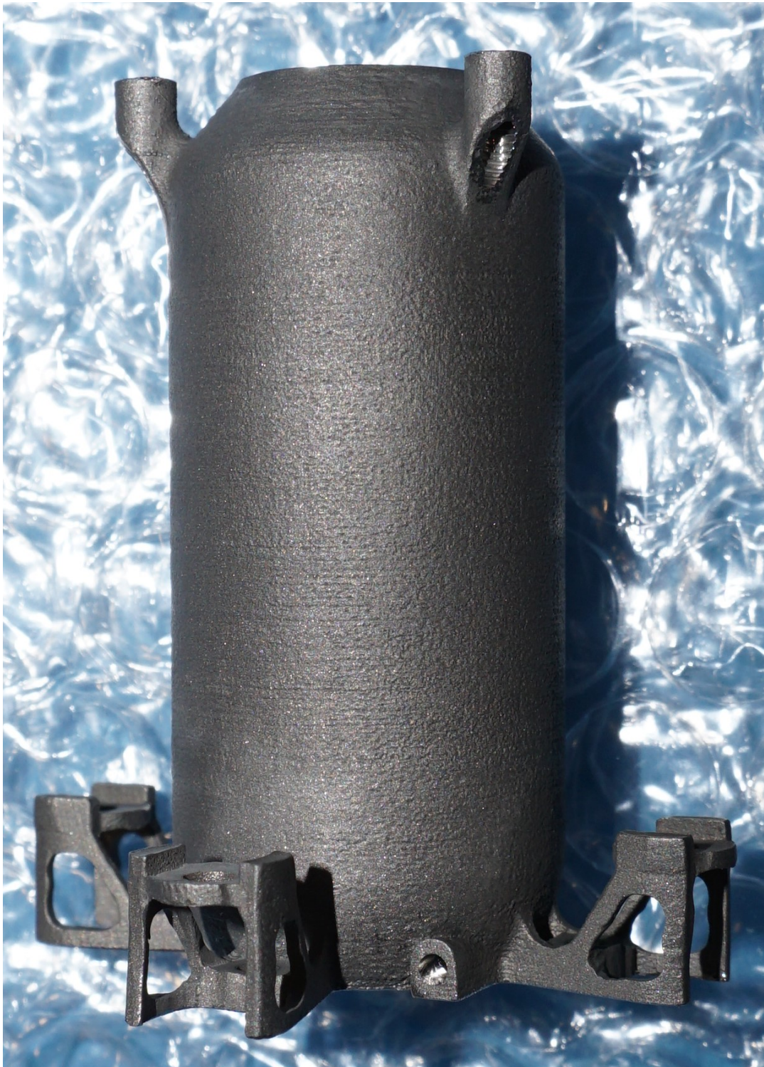
Figure B.1: AM heating chamber prototype before the integration of the nozzle and cartridge heater
