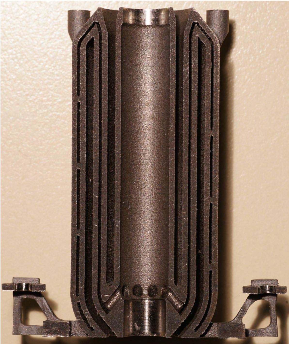
Figure B.2: Sectioned heating chamber used to inspect the capability of the printing process to accurately reproduce the inner features
