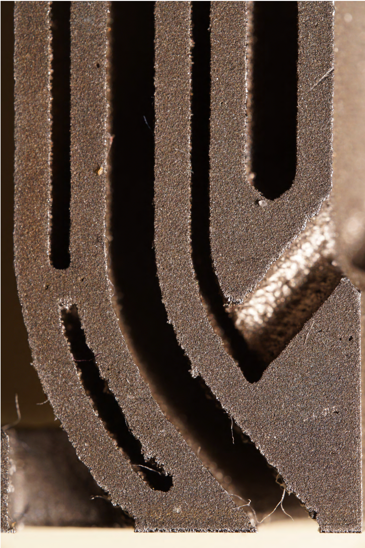
Figure B.4: Close up picture of the overhanging channel wall showing a minor print defect
