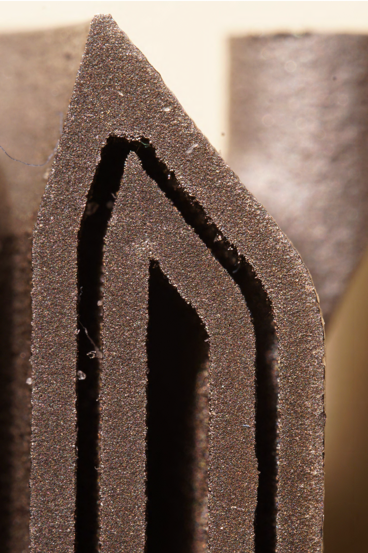
Figure B.3: Close up picture of the partially collapsed horizontal area at the transition from the first to the second channel
