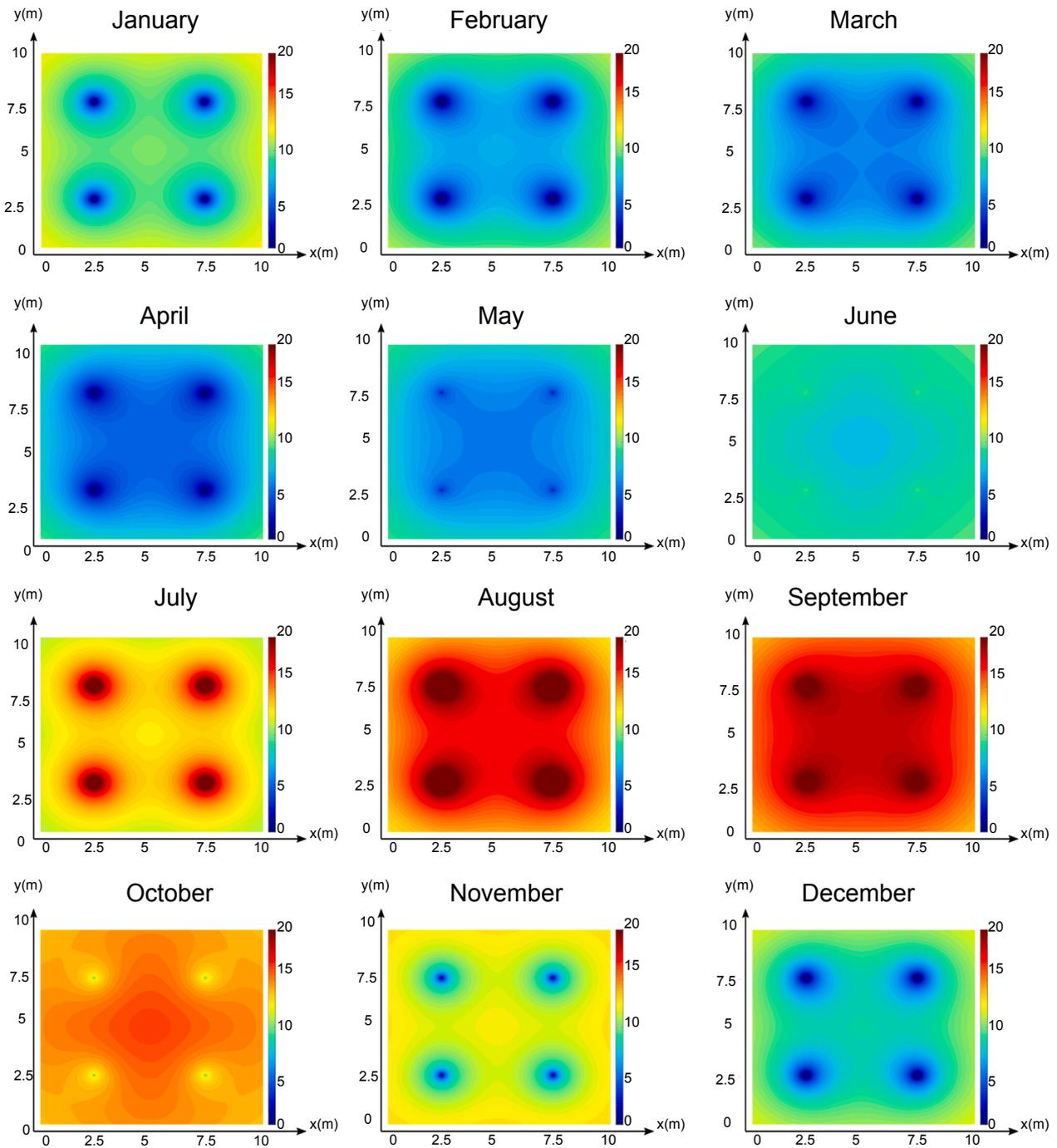
Fig. 11. Soil temperature snapshots at  $z = 100$  m for Case 2.
