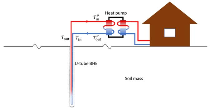
Fig. 1. A schematic representation of a GSHP system.
