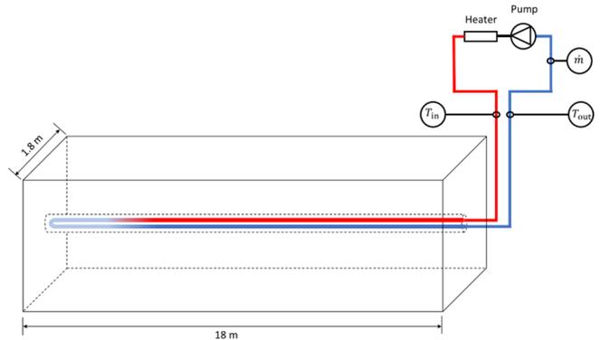
Fig. 2. A scheme of the prototype GSHP experiment, conducted by Beier et al. [26].
