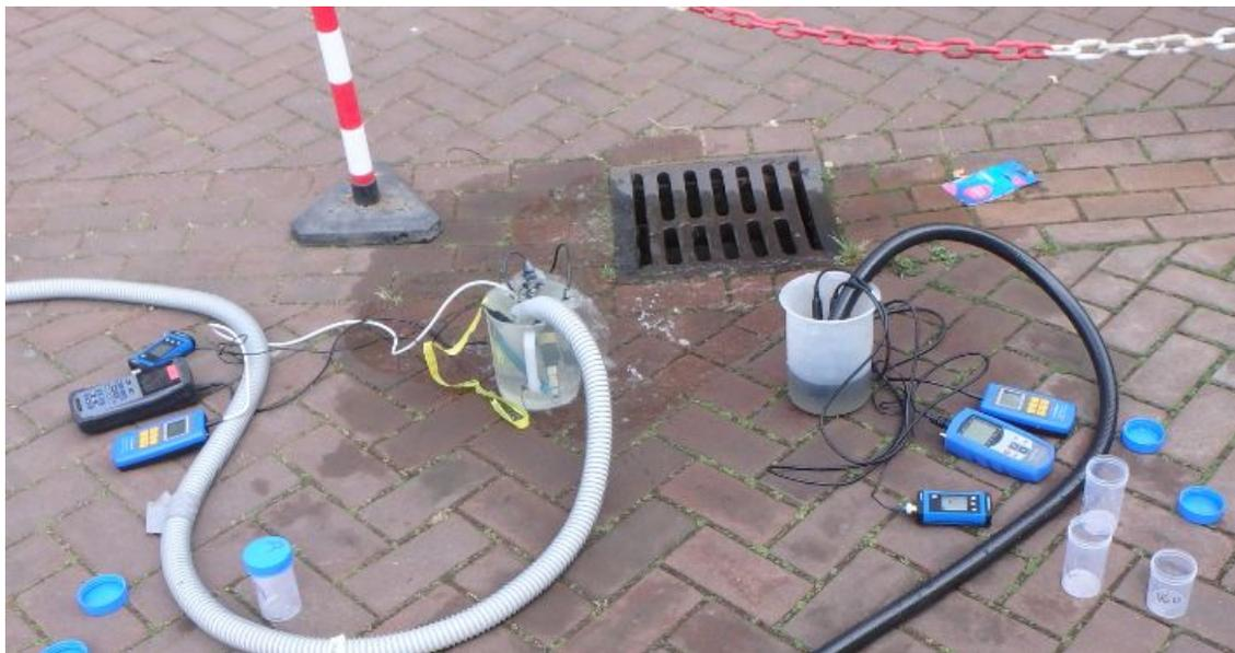
Figure 16: Two flow-through cells to measure pH, DO, EC and temperature in the water at the inlet and outlet
