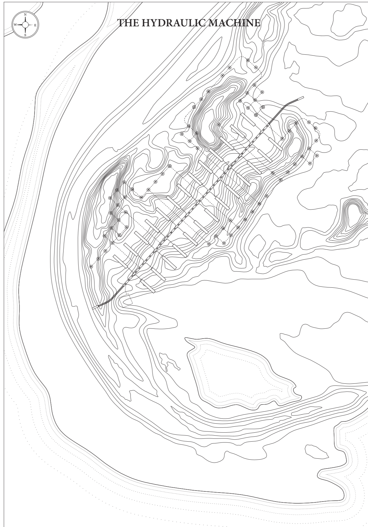
2 The Hydraulic machine produces fresh water by using freshwater lenses that are formed under the dunes of the Schiermonnikoog.
