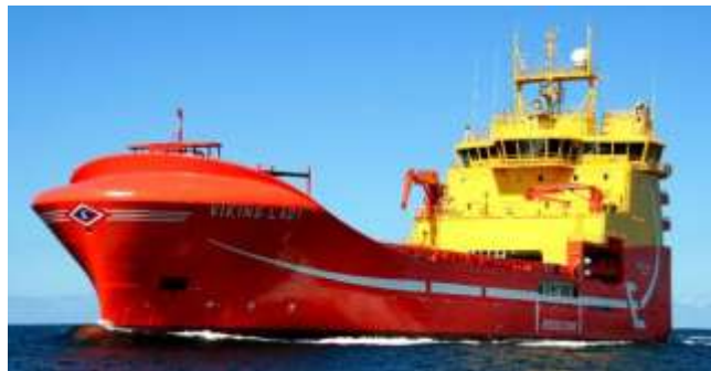
Figure 77 Viking Lady is the world's first hybrid OSV and also the world's first merchant vessel using FCs.
