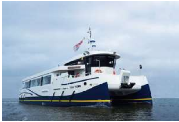
Figure 15 Ar Vag Tredan is a zero-emission electric ferry using supercapacitors [Property: STX France]
