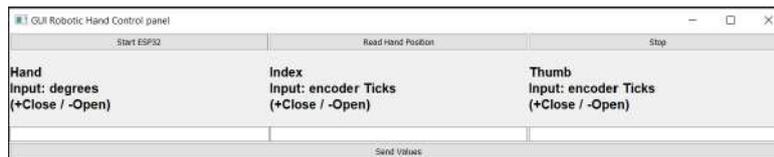
**Figure 3.23:** Graphical User Interface for the control of the prototype. Multiple buttons to start, read current position, stop, and send required positional commands using three text boxes to finely adjust values.
