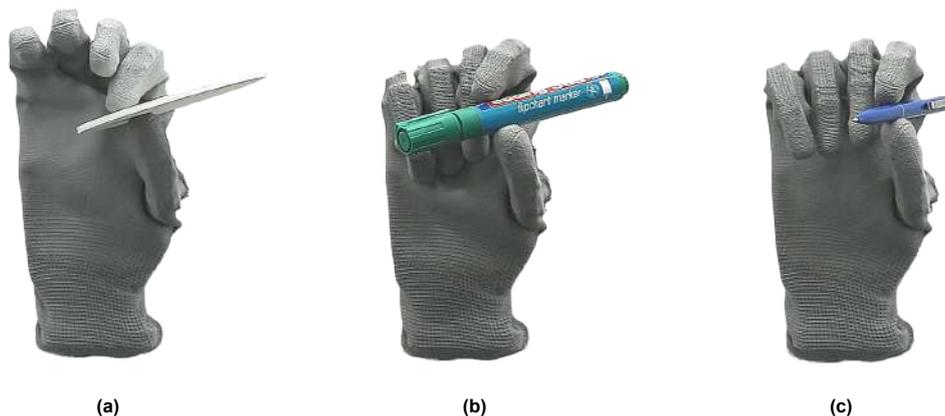
**Figure 4.9:** Grasping objects using open pinch: (a) disk; and closed pinch: (b) Marker, (c) Pen.
