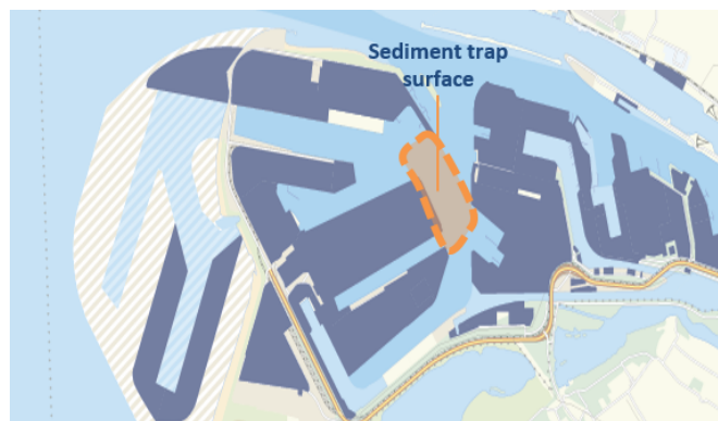
Figure 5.4: Recommended area regarding the location of a sediment trap at CaBe-MV1
