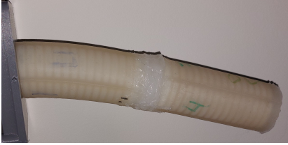
Fig. 6: Maximum gravitational torque is applied in the \theta direction by holding the robot horizontally. This results in a bending angle of approximately 15 degrees.
