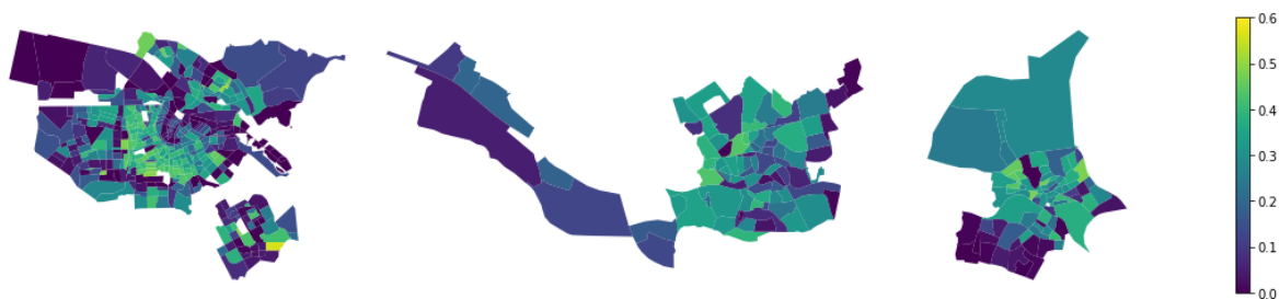
Figure 12.15: Average improvement of suitability for LT systems by insulation investment. Fltr: Amsterdam, Rotterdam, and Arnhem
