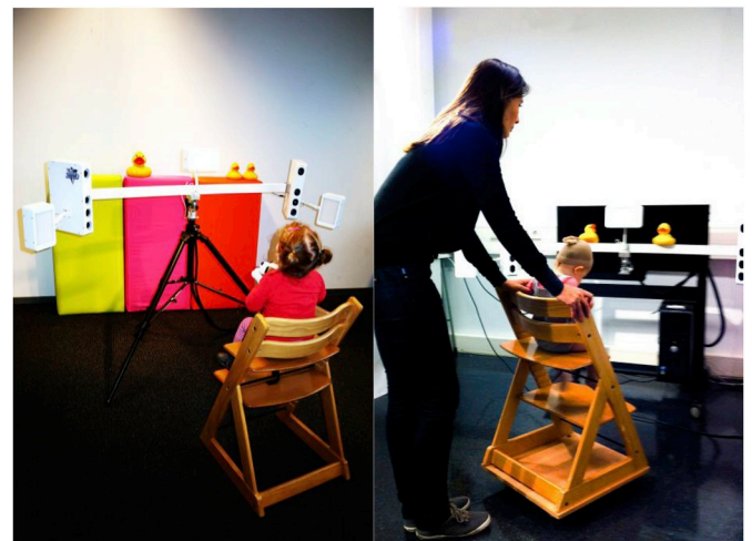
Fig. 3. 3D imaging setup with a 3-year-old girl (left) and with a 1-year-old girl sitting on the highchair mounted on the wheeled plateau (right).
