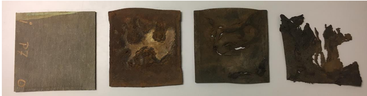
Figure 11 Rail pads in different states of decay (MOOC - TU Delft, 2021)
