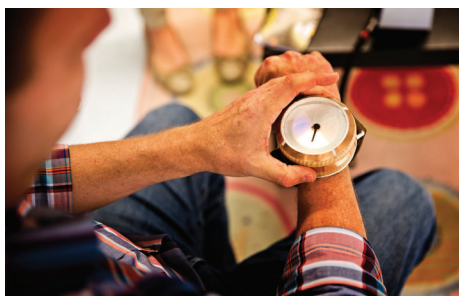
Figure 33. The exact time is not immediately apparent on Unwind. After touching the bronze bezel several times, the precise time reveals itself, while also imparting traces of our engagement with the watch and time itself onto Unwind's form. Image: Guus Schoonewille
