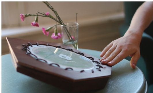
Figure 28. Phonos is adjusted by changing the positioning of the speaker itself. Moving the speaker causes a laser underneath the surface to change location, thus etching a pattern into the removable thermochromic paper that covers the surface of the speaker. Image: Aafke Croockewit, Jet Gispen, Luis Herrera, Sietse Taams, and Xi Xu.
