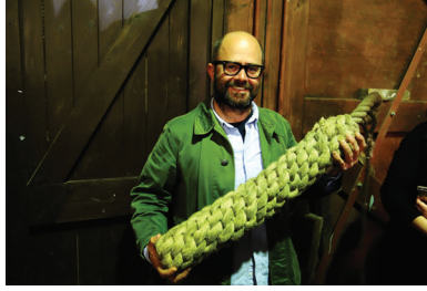
Figure 37. Rope is repurposed when it is too weak to perform a vital function on the ship and woven into a buoy to line the edge of the ship to protect it from scratching the dock. Image: Peter Bihl
