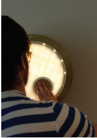
Figure 27. The outer rim of the Aila lamp is wound to generate energy for the lamp. The outer ring of lights indicates how much energy has been stored, which can be dimmed or brightened by rubbing the inner circle as demonstrated in the picture above. The wood and bronze develops patinas referencing the occasions that we collaborated with the materials to operate the lamp. Image: Jaqueline van 't Hof
