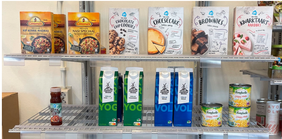
Figure 7.15: shows the setup of the shelf during all the pipeline tests. Some products have counter-parts in the setup that look similar to the desired products. Other products have multiple instances of them available to pick, forcing the robot to decide. Products differ in size and shape to test their influence on the grasp success rate.
