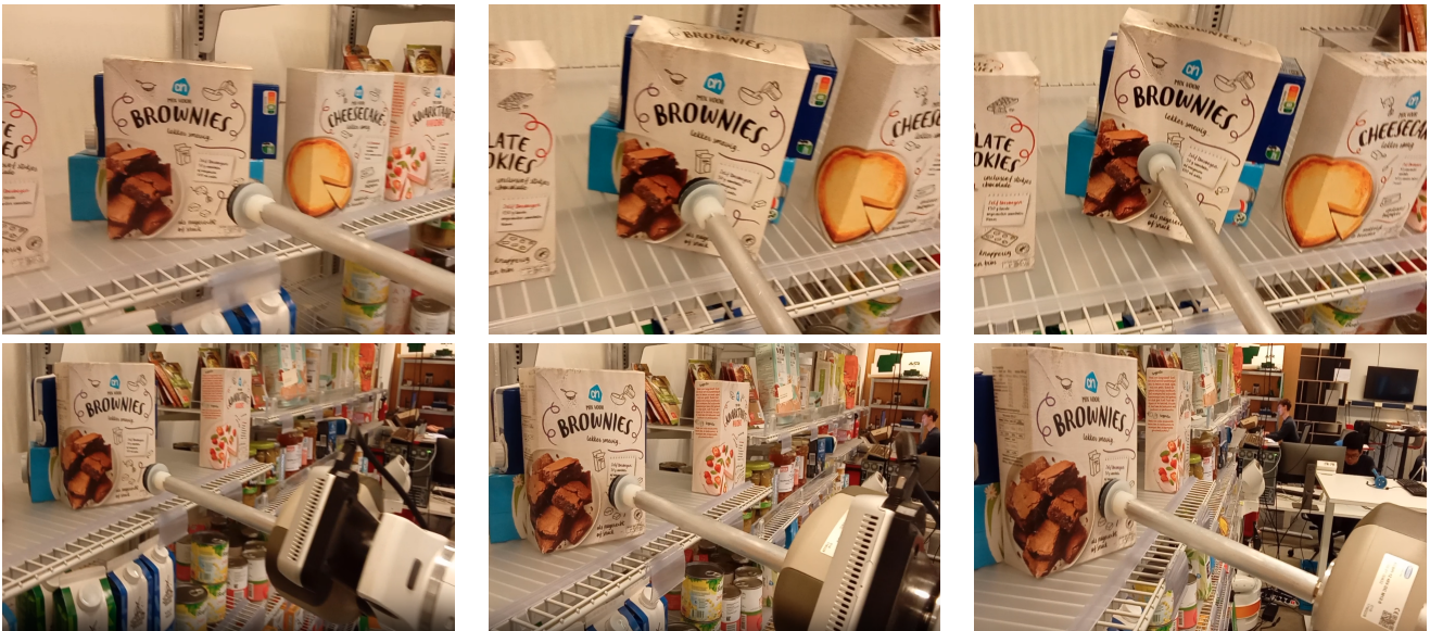
Figure 7.17: shows grasp examples without orientation estimation (top) and with orientation estimation (bottom). Although both grasps are successful, the grasp with orientation estimation managed to not deform the product and relied less on the flexibility of the suction cup.
