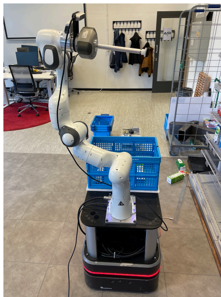
Figure 1.2: shows an image of the supermarket robot 'Albert', with the Franka Emika Panda robot arm, realsense D435i, and suction cup gripper.
