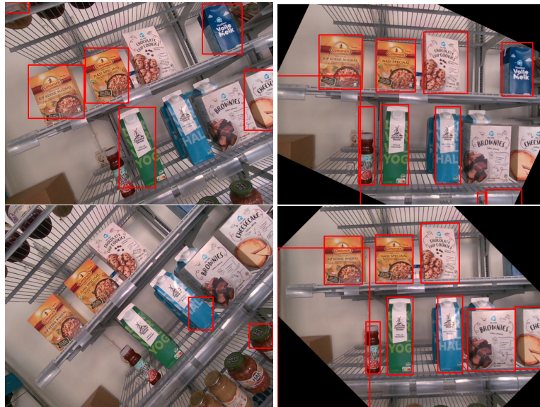
Figure 6.4: shows the effect of rotation compensation on product detection during Inference. The left images are not compensated, and the right images are. The upper images show a rotation of approximately 30^\circ , while the lower images show a rotation of approximately 45^\circ . Between left and right it can be seen that some products do not get detected at all on the left and that those that get detected have overestimated bounding boxes due to the rotation. Rotation compensation mitigates both problems.
