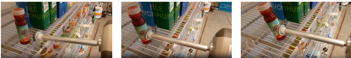
Figure B.5: shows an example of picking the 'Sweet Sour' product. This product is too light to grasp with the current suction gripper due to the low vacuum power.
