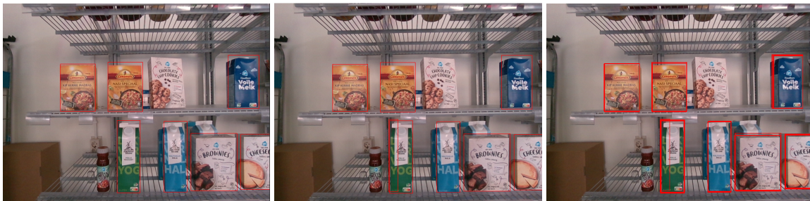
Figure 6.3: shows the effect of Non-Maximum Suppression on product detection during Inference. The left image shows an IoU threshold = 0.1, the middle image shows an IoU threshold = 0.7, and the right image shows an IoU threshold = 0.99. From right to left it can be seen that fewer proposed bounding boxes remain.
