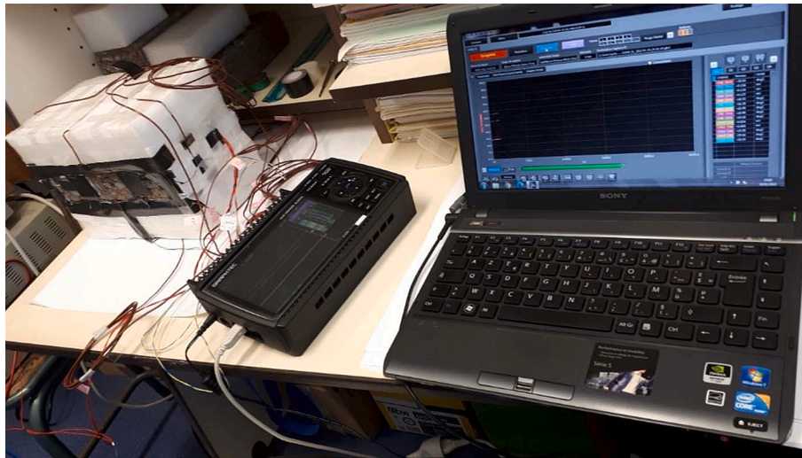
Fig. 6b. All the equipment making up the experimental measurement chain. sample, acquisition unit and computer.
