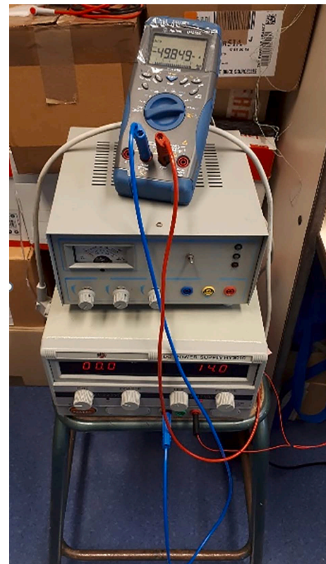
Fig. 6a. Current generation system for the heating film.
