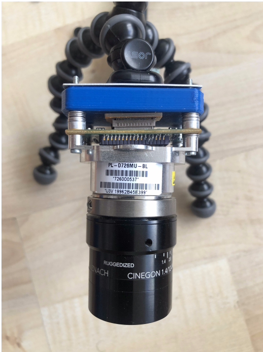
(a) Shims added on one side of the camera
