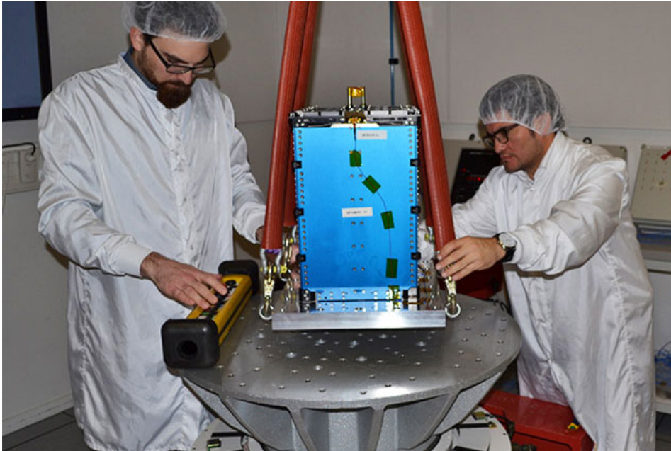
Figure 2.3: Satellite being prepared for vibration testing at ISIS [17]
