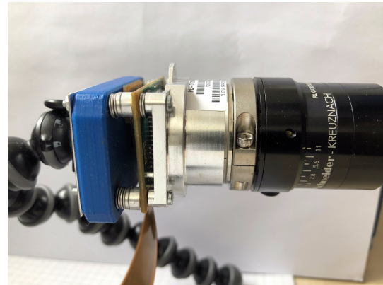
(b) Shims added on top side of the camera
