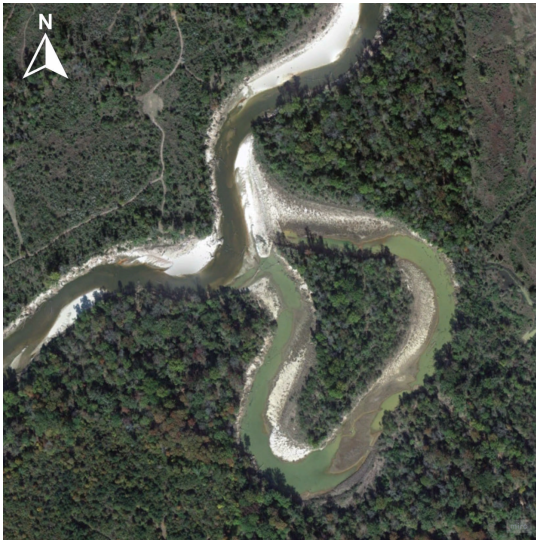
(a) Example of a neck cutoff, number 1 in Pearl River, Mississippi. The flow direction is from North to West. Image taken from Google Earth Pro, image date: 5-11-2011, near coordinates 32.111839, -90.115159.
